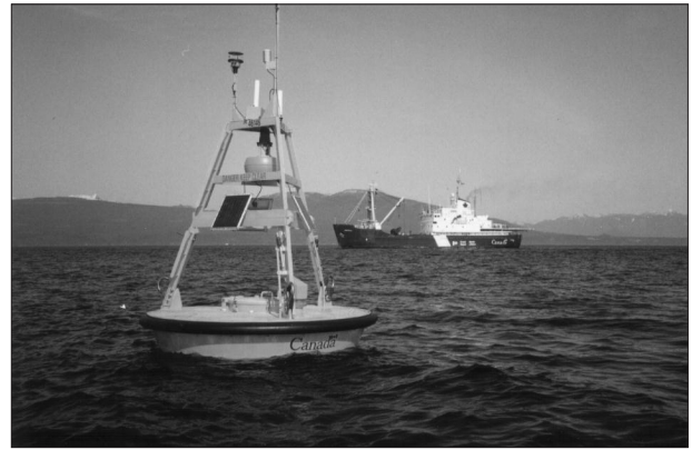
Sonic Anemometer on a buoy, Halibut Bay
