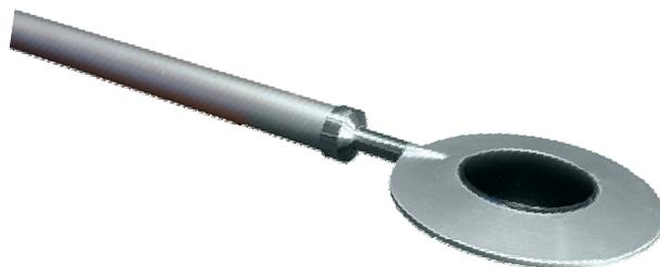
*Sensor for the measure of the **Net Solar Radiation** (Net-Radiometer) with **thermopile**. Thanks to the particular construction techniques, is able to measure the **difference between the radiation reflected from the ground and the global radiation by the sun (direct + diffuse)**.*
